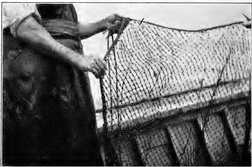
FIGURE 2.—Composite net showing differences in fouling on test panel near a pound net. The strip nearest the fisherman's hand is tarred; the others are treated with cuprous oxide treatments
